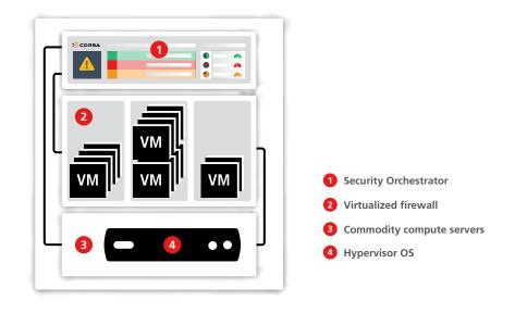
Figure 1: A turnkey virtualization platform for automating firewall virtualization
